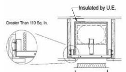
Dampers greater than 110 sq. in. are shipped with insulation factory installed on blades and box.
